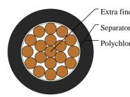
Extra fine bare copper conductor Separator Polychloroprene rubber jacket
